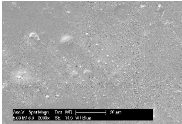
Un-Used VR™ at 2,000 Magnification
